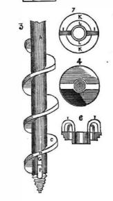
This is the invention of Mr. William Ash, of Sheffield, England. Its object is to produce holes of various diameters by one instrument by having the cutting and guiding parts detached, so as to change them at pleasure. Figures 1, 2, 3, represent the augur in three
