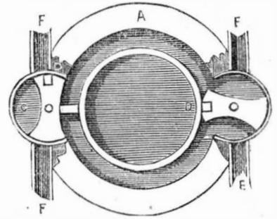
side of the engine, by a spindle passing through the top. D is a piece of chilled iron in the cock to resist the friction of the revolving cylinder, as explained in last figure. E is the steam passage and F the passage to the condenser.
