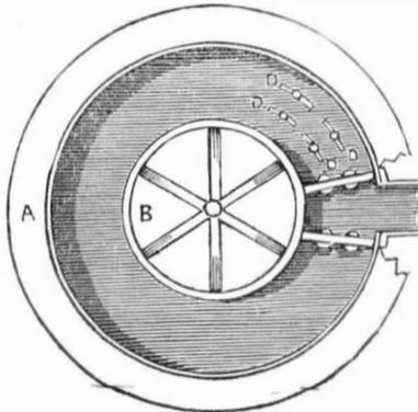
A is the outside fixed cylinder. B, the inner or revolving cylinder, D D, two or more pallets working through a deep stuffing box, and turned by a lever or other power from the external part of the engine alternately flat or edgewise; the pallets D D, are fixed to the revolving cylinder, E is the steam passage—the one to the condenser is not shown.
