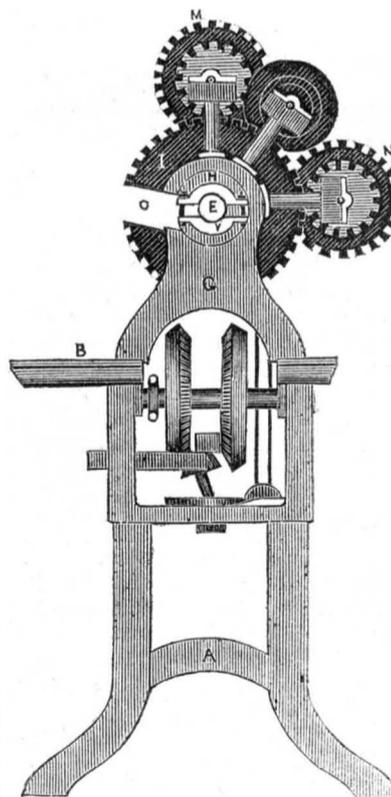
pin projecting into the slot of the chuck, when the chuck will be revolved the axle will thus be revolved with it.
