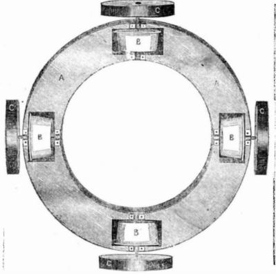
The above engraving represents the application of horse power in a very diversified manner by friction rollers on which there is a top circular rail for the horse or horses to be attached by levers, and which rail is left out of the engraving to show more clearly the interior working of this machine, so well adapted to so many purposes.
