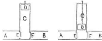
upon all sides, the pressure upon E will be that due to the steam, and will be, if there is any truth in theory, a propelling power. I confess I am unable to see that the whole of the pressure of the steam down to the atmospheric point, is not effective power. If not—why not? If it is—why is it not the best of all possible methods?
